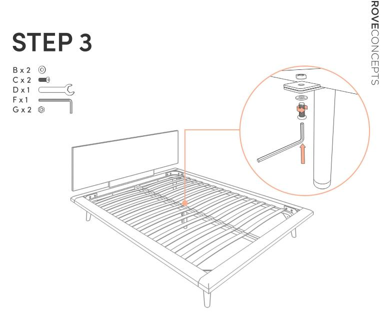
• Combine "B", "C", and "G" to attach center leg to slat frame
